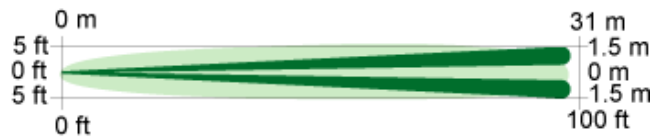
Top View Optional Long Range Coverage: 30.5 m x 3 m (100 ft x 10 ft) Requires optional ORL92-3 lens.
